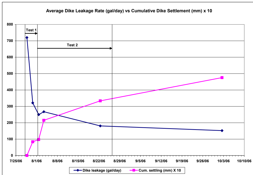
Figure 26. Plot of dike leakage and dike settlement over time.
