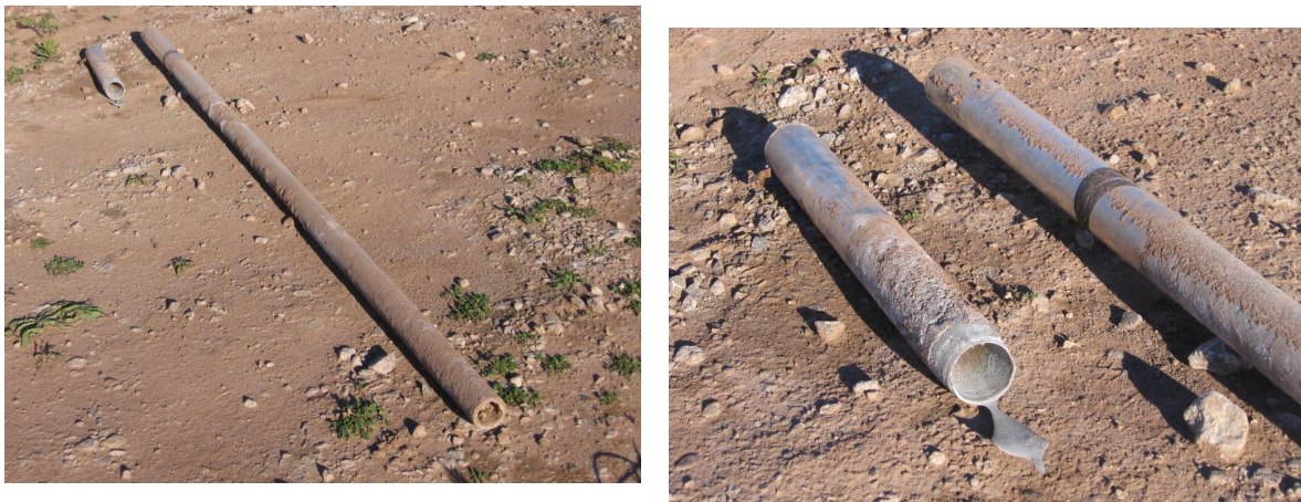
Figure 39. Depleted aluminum anode compared to an intact anode.
